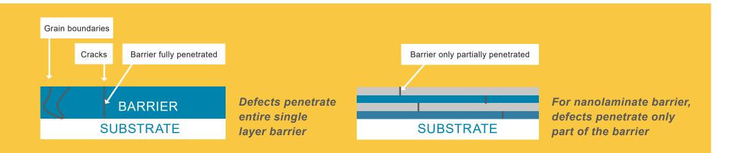
Multilayers reduce both crack and grain boundary formation, reducing the number of active diffusion paths.
